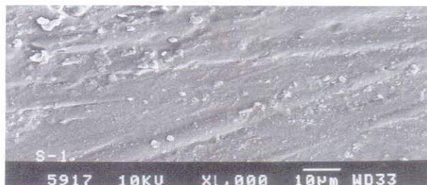
Fig. 1 SEM of polyurethane nanocomposite samples containing 2 wt% of nanoclay
