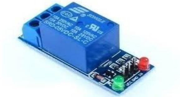
Fig1.8: Relay Module
