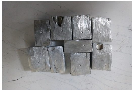
Fig. 5. Specimen for hardness test with hardness testing machine
