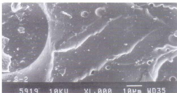
Fig. 2 SEM of polyurethane nanocomposite samples containing 1 wt% nanoclay
