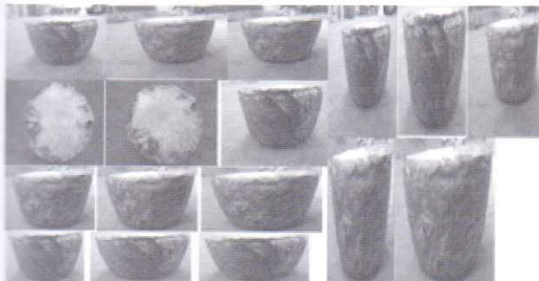
Fig. 2 Produced 17 pieces of Metal Matrix Composites (C355+5%SiC)
